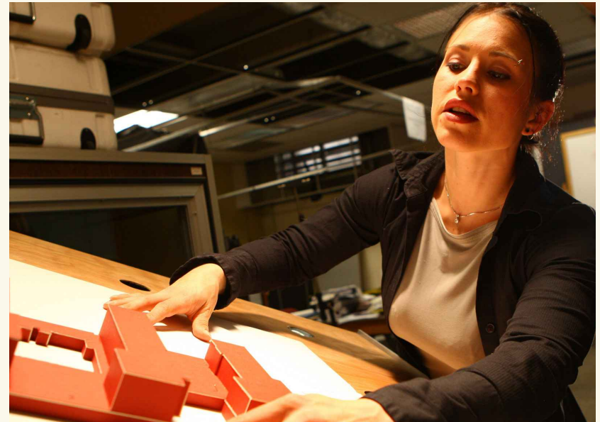
Gwynne Mhuireach uses a heliodon to analyze how sun and shade would affect the outdoor spaces around a building as part of her work as the SRG Partnership Graduate Research Fellow in Architecture.
